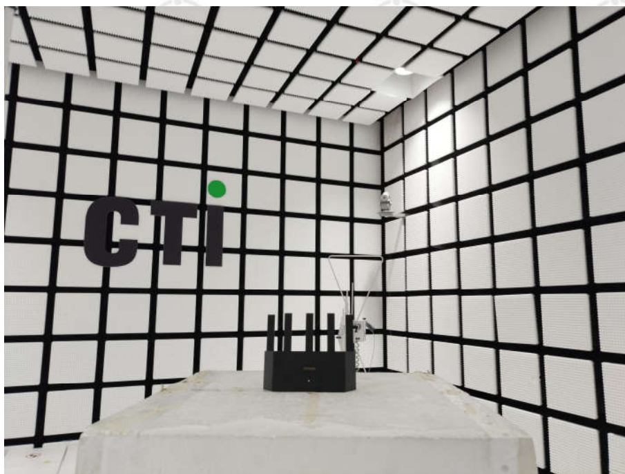
Radiated spurious emission Test Setup-1(Below 1GHz)
