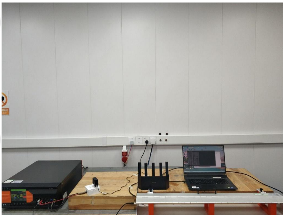
Electrical fast transients burst Test Setup-2
