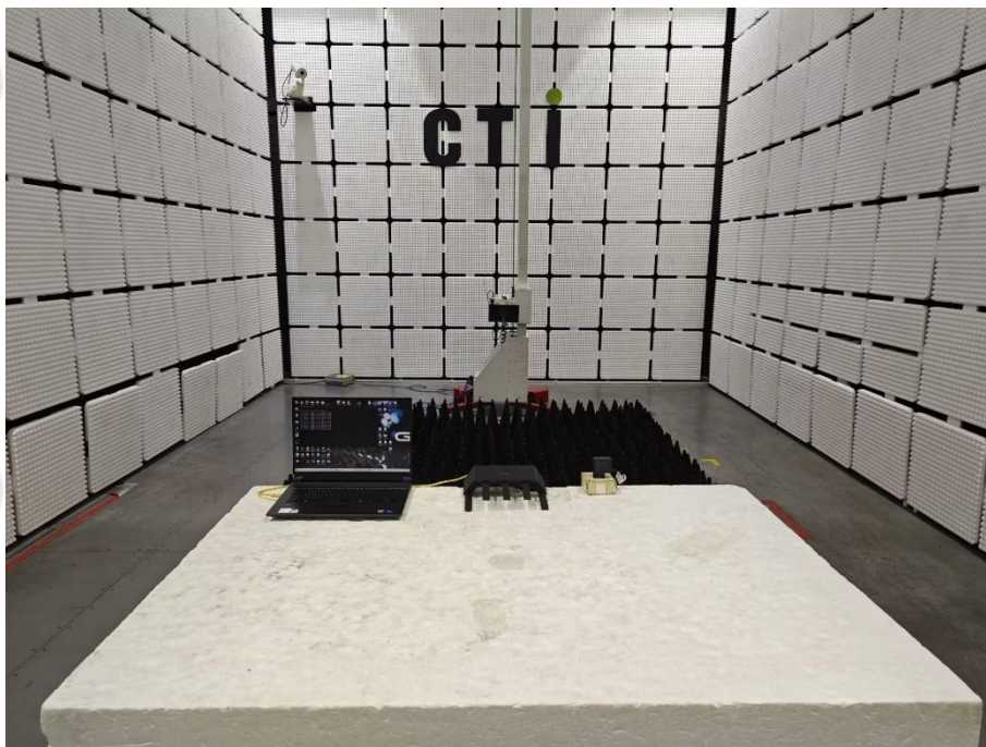
Radiated emissions Test Setup-2
