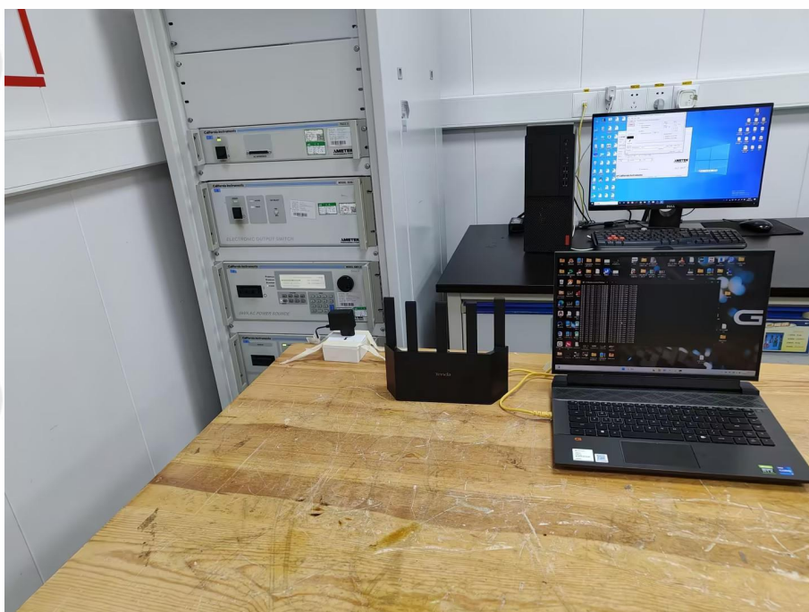
Voltage dips and interruptions Test Setup-2
