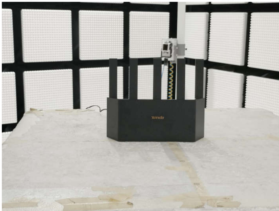
Radiated spurious emission Test Setup-3(Above 18GHz)
