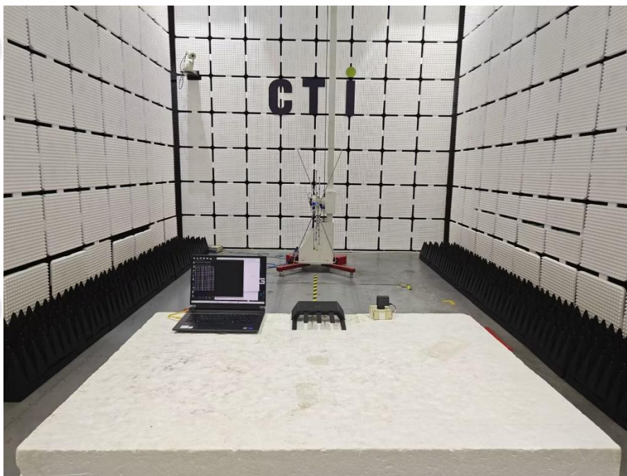
Radiated emissions Test Setup-1
