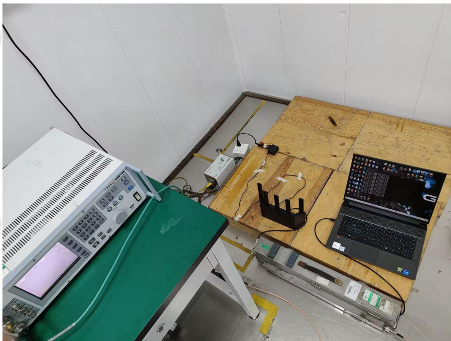
Continuous induced RF disturbances Test Setup-3
