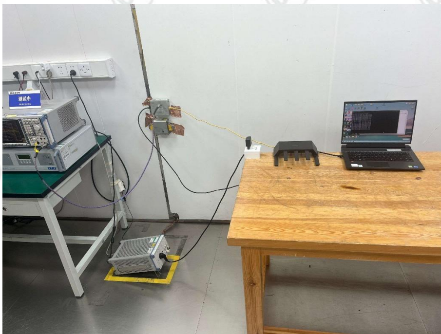
Conducted emissions Test Setup-1
