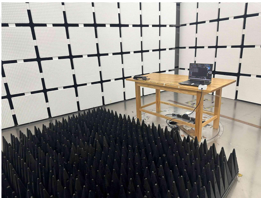
Continuous RF electromagnetic radiated field disturbances Test Setup-1
