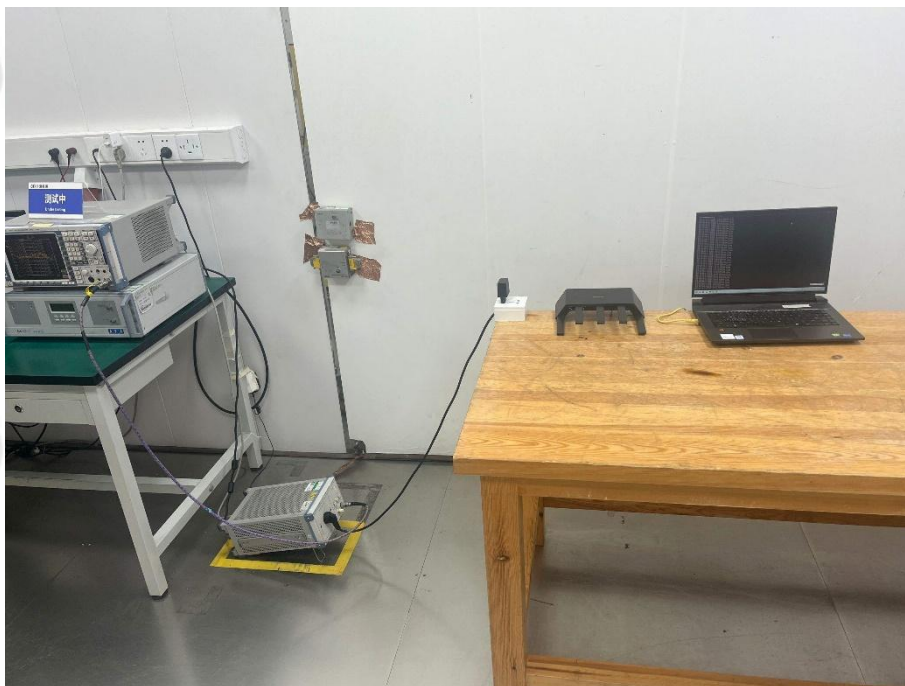
Conducted emissions Test Setup-3
