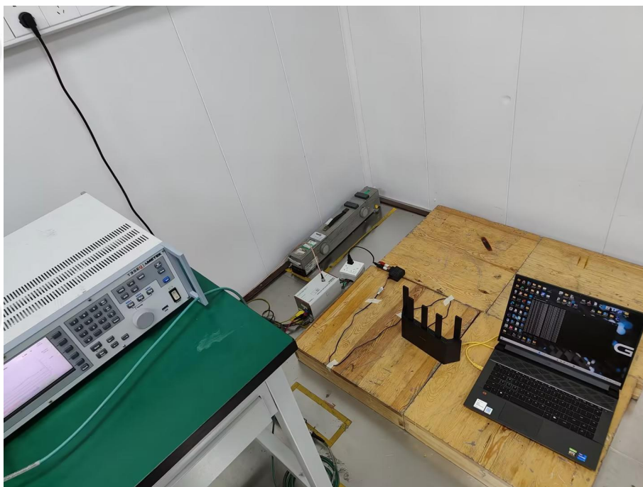
Continuous induced RF disturbances Test Setup-1
